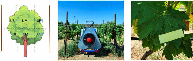
Figure 11 The effectiveness of the autonomous spraying system in table grapes was assessed in the field using strips of water-sensitive paper. See main text for explanation.
