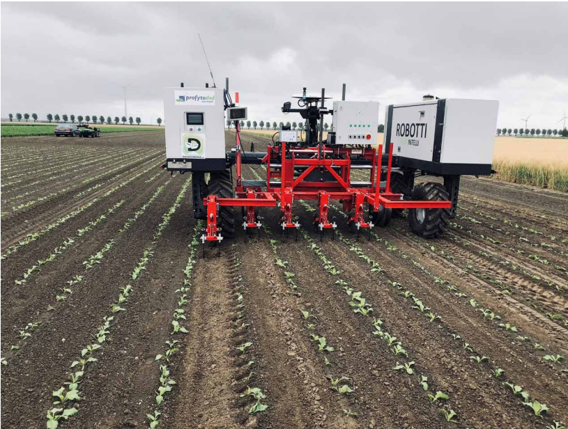
Figure 4 The weeding implement used in the pilot in the Netherlands, mounted on the Robotti robot.
