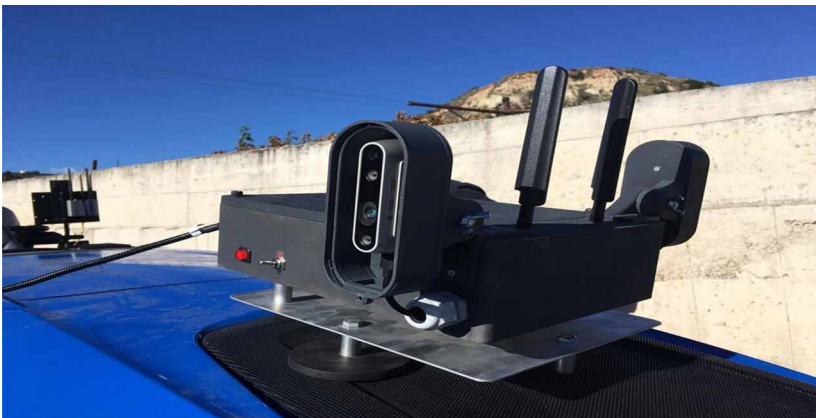
Figure 10 The canopy density perception unit mounted on the hood of the tractor. The unit has two depth cameras (RealSense D435i, Intel, Santa Clara CA, USA) (one camera is facing the viewer). Also visible are two antennas for the wifi router that is part of the unit.
