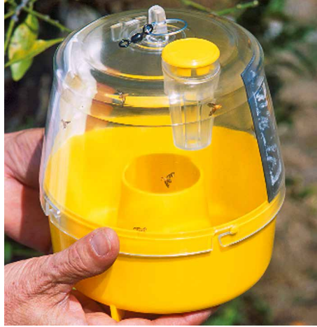
Figure 9 A McPhail trap for monitoring fruit flies (Tephritidae). Flies enter the trap through an inverted funnel entrance in the bowl base attracted by pheromone lures or liquid food baits. Source: Image by Peggy Greb, USDA Agricultural Research Service.
